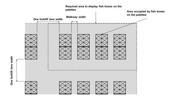
Figure 8.5 Example of arrangement of fish boxes on the palettes in the auction area
