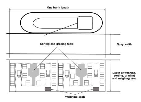
Figure 8.3 Example of arrangement of sorting tables for one berth
