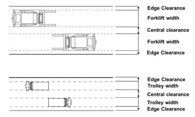
Figure 8.8 Forklift lane and trolley lane
