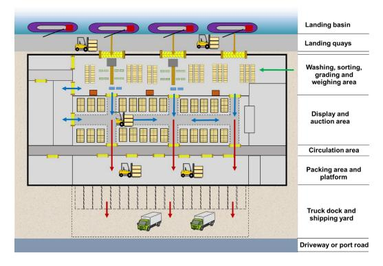
Figure 7.5 Image of use of areas and flow of fish and fishery products in the main building
