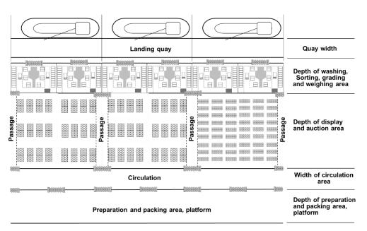
Figure 8.7 Example of arrangement of circulation and passage
