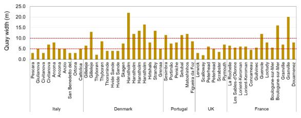
Figure 8.1 Example of landing quay widths by country and fishing ports
